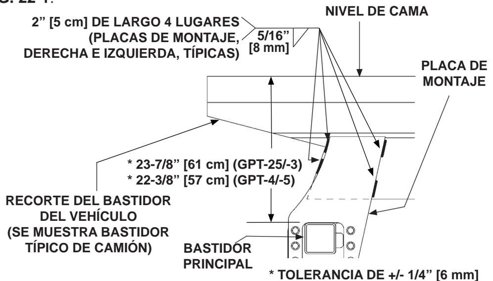
**SOLDAR AL BASTIDOR Y AL BASTIDOR PRINCIPAL (SE MUESTRA LADO DERECHO)**
