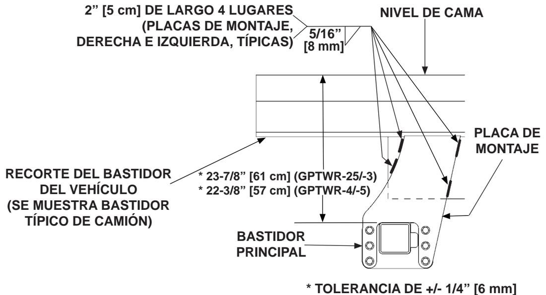
SOLDAR AL CHASIS Y AL BASTIDOR PRINCIPAL (SE MUESTRA LADO DERECHO)
