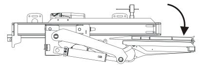
No contact between slideframe and platform
