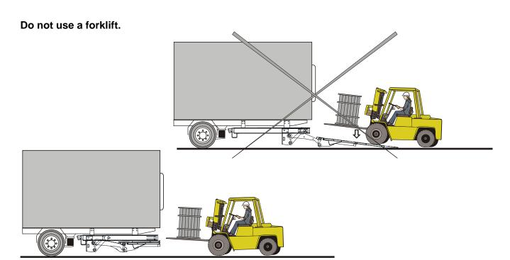
Only when the Slidelift is retractet under the vehicle.
